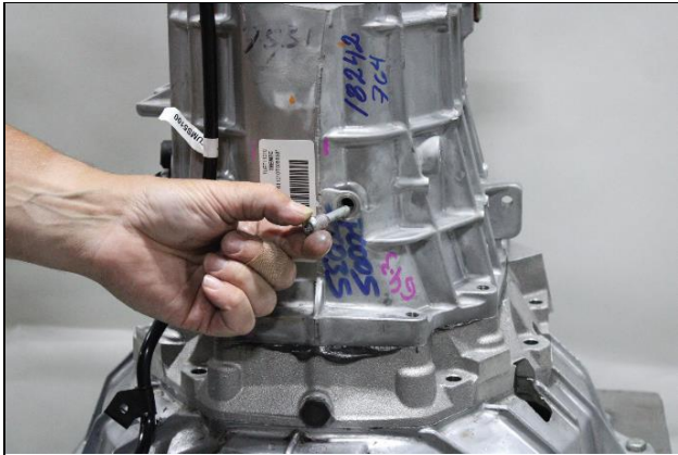
8.18: Install 2 shift linkage locating bolts into case using a T 40 bit.
