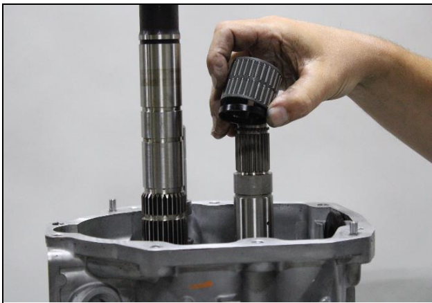
8.22: Install 6 th gear needle bearing onto countershaft
