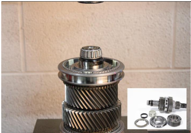
6.6: Using a press install 3 rd gear blocking rings, bearing and gear onto main shaft, Careful to align blocking rings into synchronizer as you press onto main shaft.
