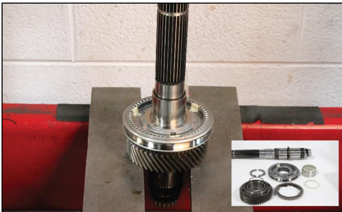
5.6: using and press and main shaft support remove 2 nd gear 1-2 synchronizer, bearing and blocking ring assembly.
