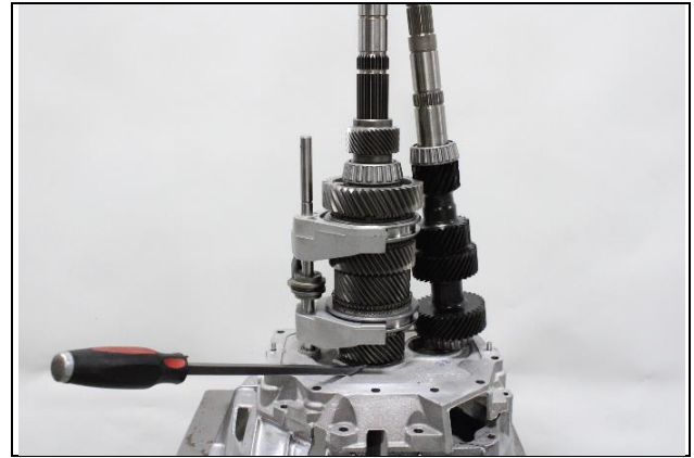
8.12: Using and prybar or large flat screwdriver gently lift main shaft assembly upwards to allow counter shaft room to fall not midpalate bearing race.
