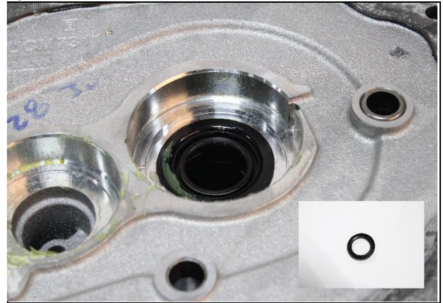
3.33: Remove 4 th gear "Input shaft" transmission seal from Mid plate.
