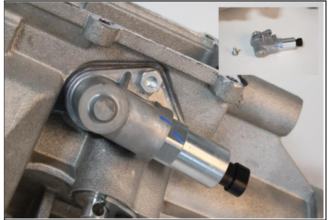
4.2: Remove 13mm Bolt from rear housing.
