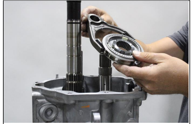
8.25: Install 5-6 synchronizer and fork on to main shaft.
