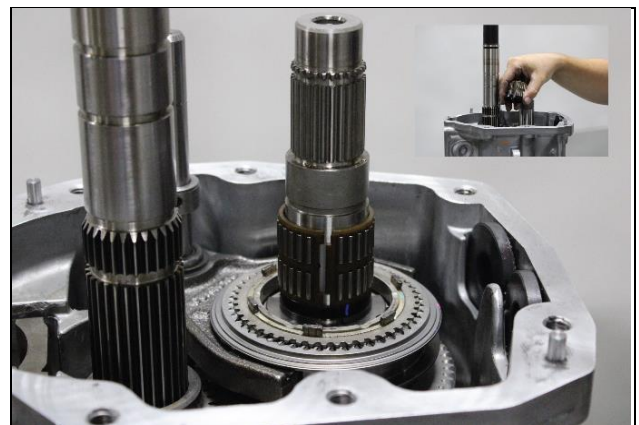
8.29: Install 5 th gear thrust washer and roller bearing onto counter shaft.
