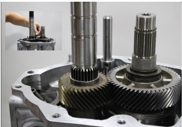
8.34: Install 5 th drive gear split washers onto main shaft.
