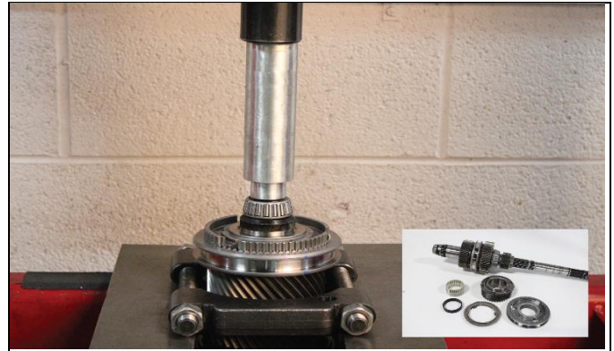
5.2: Using a press & Press plate remove 3-4 synchronizer while supporting 3 rd gear.
