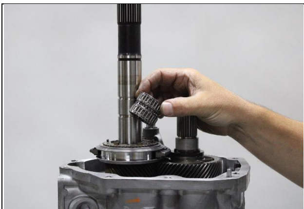
8.40: Install reverse gear roller bearing.
