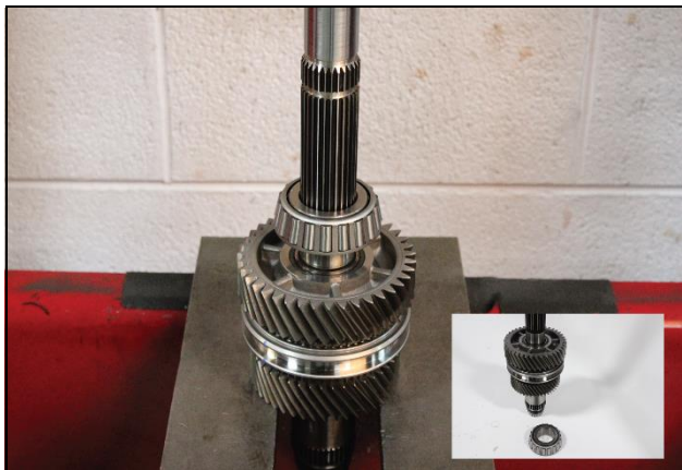
6.4: Using a press install main shaft Roller bearing.
