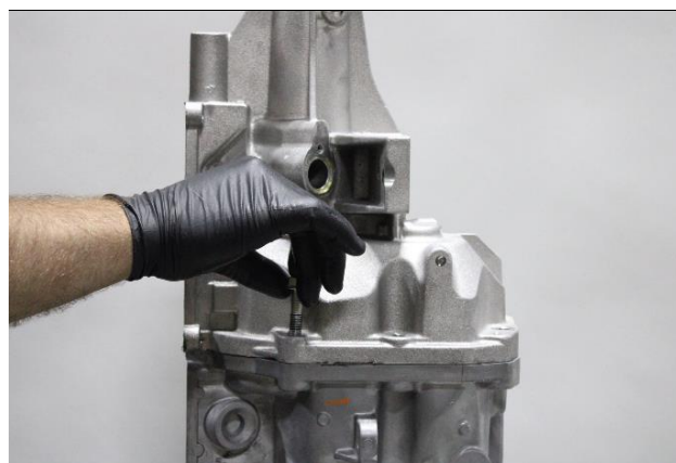
8.54: Install 8, 15MM Bolts into rear housing.
