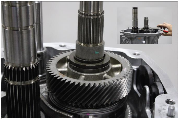
8.32: Install rear housing and shift lugs together on transmission
