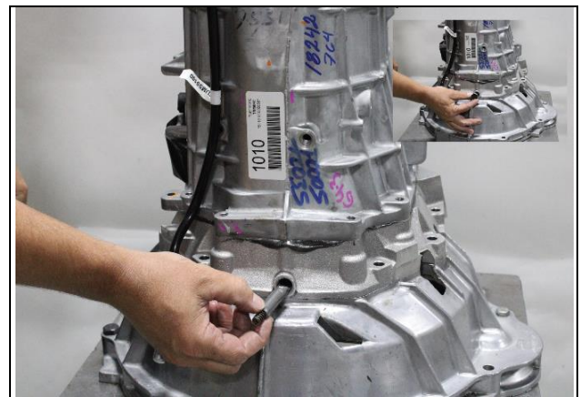
8.17: Install detent spring and plunger into case.
