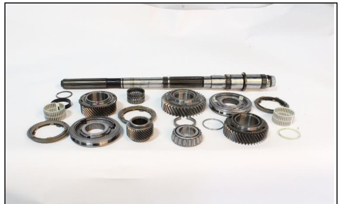
5.7: With main shaft disassembled clean all components for inspection.
