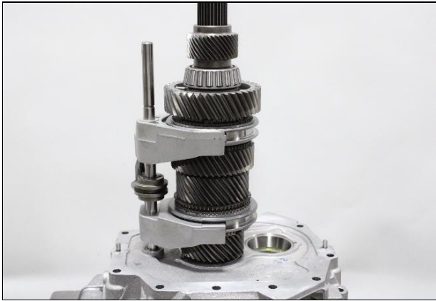
8.11: Install Main shaft assembly & fork assembly onto mid plate, it is important to keep synchronizers on main shaft in the neutral position for alignment of shift rail locating bolts.
