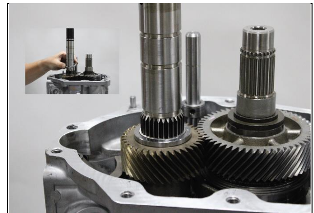
8.35: Install Locking ring onto main shaft.
