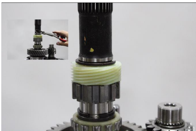
8.50: Install Speedometer gear snap ring onto main shaft.
