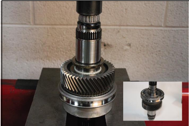
6.1: Install 2 nd gear, bearing, blocking rings and 1-2 synchronizer onto main shaft.
