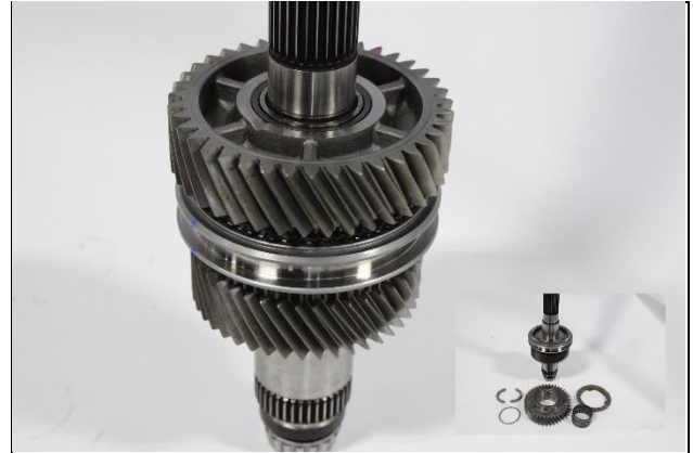
6.3: Install 1 st gear bearing, Gear and blocking rings onto main shaft. Careful to line up blocking ring tabs into 1-2 synchronizer.
