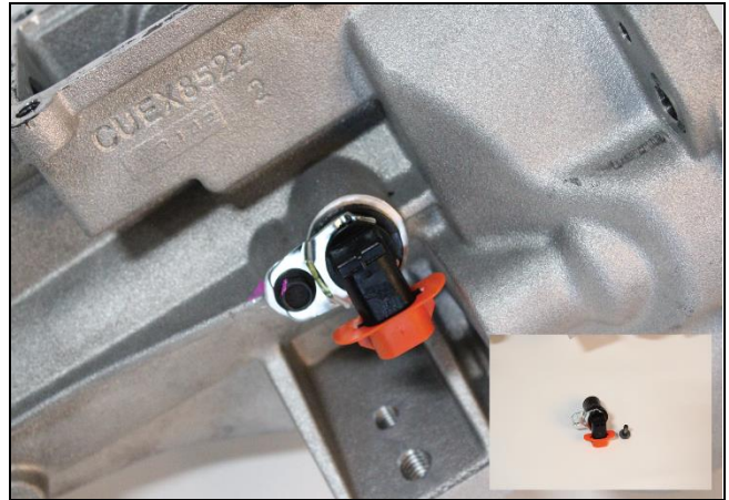
4.5: Remove 7/16 bolt from rear housing.
