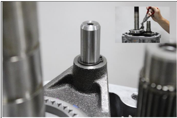
8.38: Install reverse gear fork snap ring onto shift rail, careful to seat snap ring into rail fully.
