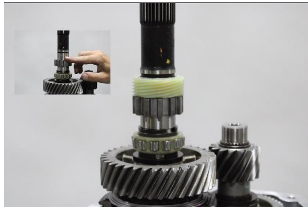
8.49: Install retaining ball into shaft and Mechanical speed gear onto Main shaft.
