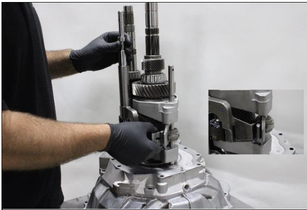
8.13: Install 5-6 & Reverse shift linkage into midpalate. Align fork into interlock on main shaft.
