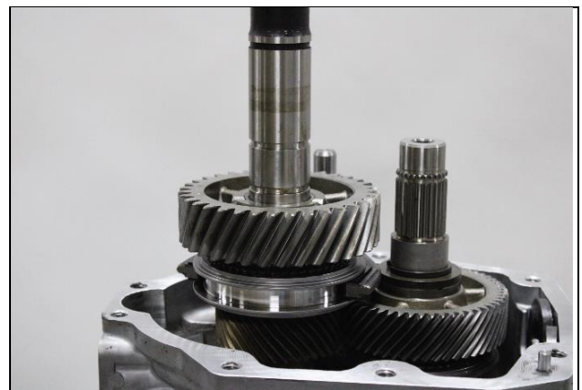
8.41: Install reverse Gear. Careful to align gear tabs with blocking ring tabs.
