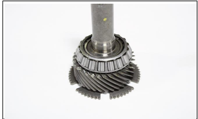
8.3 Using a press, install new Roller bearing onto input shaft.
