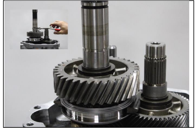
8.43: Install reverse gear snap ring.
