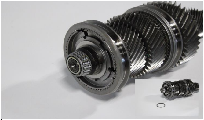
5.1: Remove snap ring from 3-4 synchronizer.
